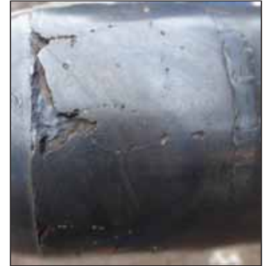
Spalled Hardbanding - Rejectable
