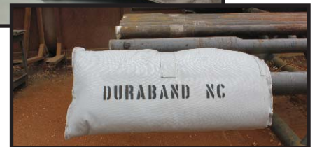
HB Insulator Bag installed on tool joint
