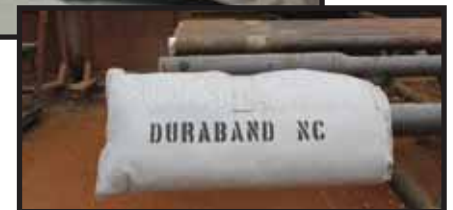
HB Insulator Bag installed on tool joint
