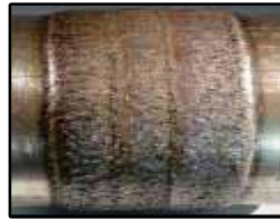
Ultraband ® NM w/ 20-30 Mesh Cast Carbide
