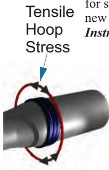
below just underneath the hardbanding. These values typically transfer to the HAZ on the surface of the tool joint, shown in Yellow on Page 1. The average in this case was 29.6 Rc. Although hoop stresses were not measured, logic would indicate that hoop stresses would be lowered as well. These factors are critical to lowering high stress sites around and including the hardbanding weld metal.
