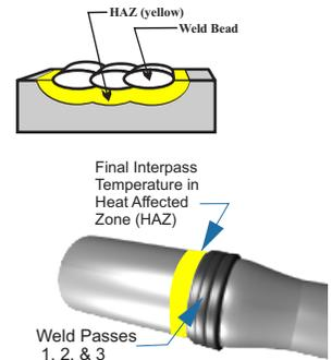
temperatures prior to hardbanding, controlling weld interpass temperatures during hardbanding, and ensuring very slow cooling procedures by deploying insulation over the weld after hardbanding.
