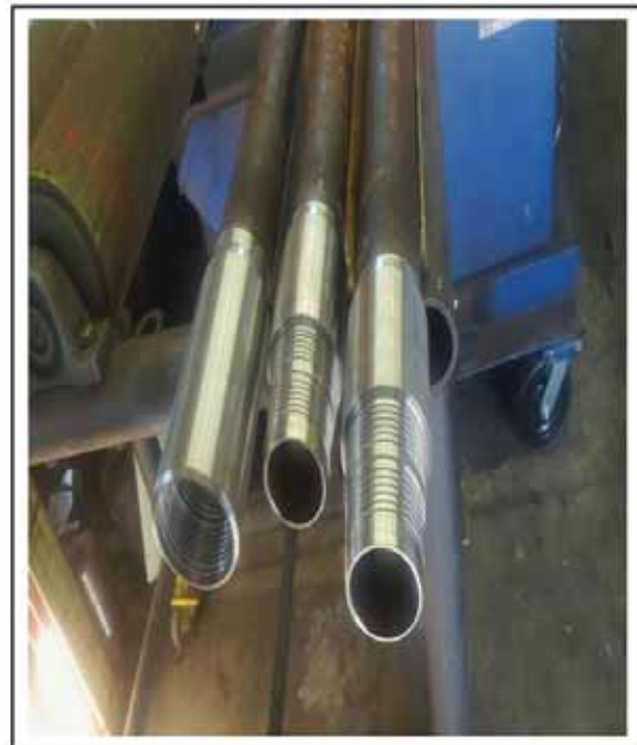
FIGURE 3B Restored Connections after Buildup Procedure
