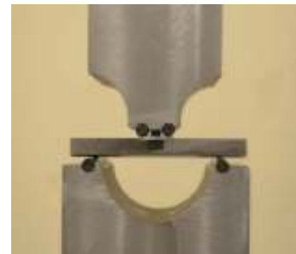
Fig. 2 A fatigue test sample mounted in the special designed fixture (4 point loading).
