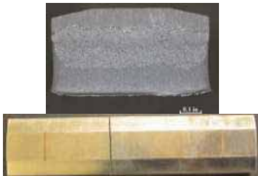
Fig.3A Duraband . The sample was brought to failure after 1,000,000 cycles. The upper photo shows the cross-section of the fractured surface. Note that there are no flaws in the weld deposit, which produces desirable fatigue failure results. The lower photo shows no flaws in the weld deposit that could produce premature fatigue failures.
