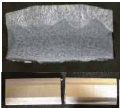
Fig.3B Tuffband . The upper photo shows the cross-section of the fractured surface. Note There are no flaws on the hardbanding surface. The lower photo shows the sample which exhibited no flaws. Tuffband was cycled beyond 1,000,000 cycles to fatigue failure.
