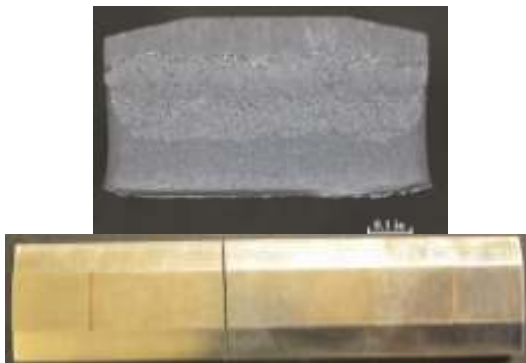
Fig. 3A Duraband® NC. The sample was brought to failure after 1,000,000 cycles. The upper photo shows the cross-section of the fractured surface. Note that there are no flaws in the weld deposit, which produces desirable fatigue failure results. The lower photo shows no flaws in the weld deposit that could produce premature fatigue failures.
