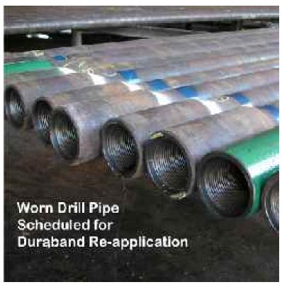
As the drilling industry evolves to accommodate the challenges of deep well and horizontal drilling techniques, more demand is being placed on the maintenance of drill strings, and in particular the tool joints. Perhaps as little as 15 years ago, tool joints were protected quite adequately by tungsten
