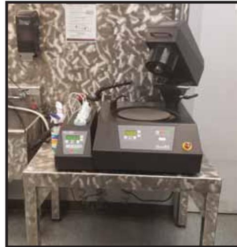
sectioned and prepared. This requires careful sectioning, mounting, and polishing with diamond particles. The sample is then etched to bring out the structure.
