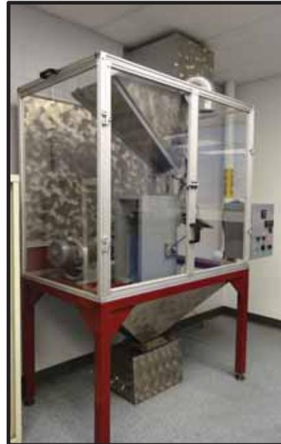
Quite simply, a test piece is placed in the holder and loaded with a 30 pound force against a rotating rubber wheel. Closely controlled sand is then trickled down between the test piece and the rubber wheel. At the end of a predetermined number of rotations, the sample is then examined for weight loss. It is this weight loss which determines the abrasion resistance of the hardbanding. These numbers are compared to other products in our massive database.
