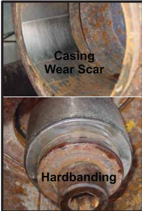
A number of very valuable parameters are derived that help describe the effects of a certain hardbanding on casing wear. One of these is the “Wear Factor” in which very low numbers are desirable. Another is the amount of casing worn in 8 hours. Again, low numbers are desirable. A third parameter is the number of revolutions that are required to remove 12.5% of the casing. In this case, higher numbers are desirable.
