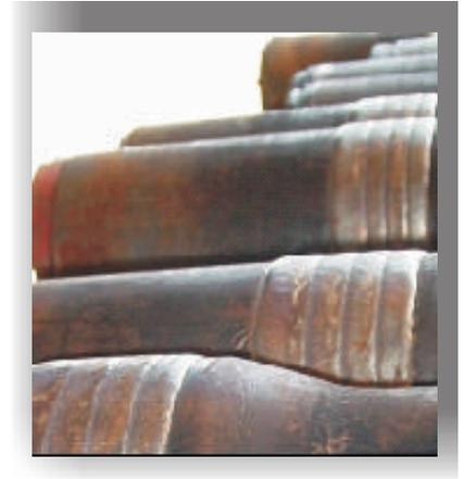
Protecting the IPC is easy. Filling the pipe with water will keep the temperature at a low enough level so as not to burn the IPC. The problem is that this would cool down the temperature in the tool joint, causing too high a hardness in the HAZ(heat affected zone)
