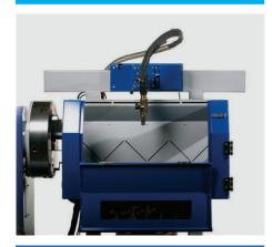
We've designed our hardbanding unit with a unique system of low and high pressure fume extraction, directed through carefully positioned vents. In factory conditions, this will remove almost all welding fumes without disturbing gas flow at the welding torch.
