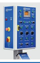
Once welding and torch positioning parameters are set, the operator simply has to select the number of bands required and press the Weld button to run the program.
