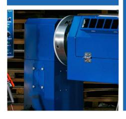
The robust three jaw chuck is made to order in the UK especially for Hardbanding Solutions. We set our chuck speed to minutes and seconds, so changing it for varying diameters of tool joint is fast and simple. It will turn at speeds from 0.2 rpm to 2 rpm as standard. If you need it higher, we can do that on request.
