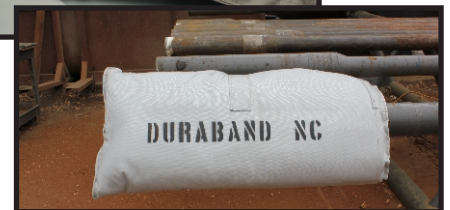
HB Insulator Bag installed on tool joint
