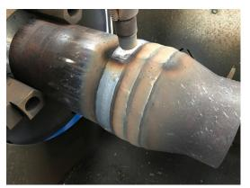
3. <u>Automatic</u> application of Duraband NC Hardbanding, 3 x 1" bands, 2.5mm height.
