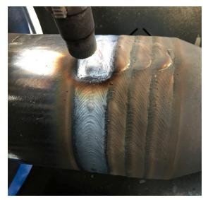
2. <u>Automatic</u> application of Postle Tool joint Build Up, 4 x <sup>3</sup>/<sub>4</sub>" bands, 2.5mm height.
